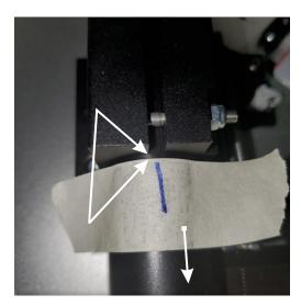
In this example, the tube has moved more closely to the core (bottom of the sensor). Pollen Sense support technicians will instruct you as to the direction the tube should move.
