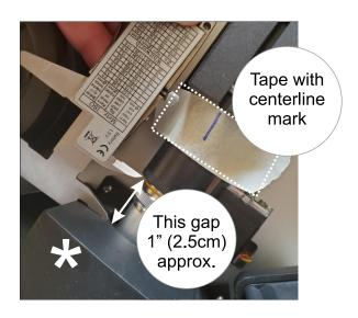
Unless the microscope tube is completely loose in its bracket, put a piece of tape with a centerline mark at the place where the tube meets the bracket. This will serve as a reference during adjustment.
