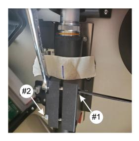
Use a 3mm allen hex wrench and a 7mm or small adjustable wrench and loosen the bolts enough that the microscope tube begins to slide in the bracket around it.
