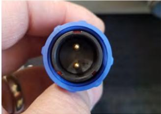
Once it's seated firmly, twist the section connected to the cord between the power supply and closest to the device until it is hand-tight. **Do not overtighten or use tools!**
